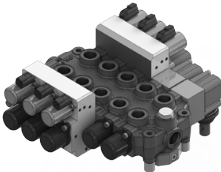
OP20 configured with 3 solenoid actuated spools with manual override and 2 manually operated spools (in the upside-down configuration). Typically utilised in Tilt Tray applications
